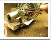
STEP 9: Connect the white wire from the LED driver to the red wire from the motor and the long red hook-up wire using a wire nut. Use a wire tie to bundle the wires as shown.
