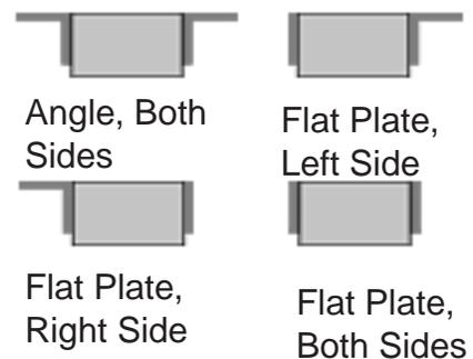
Bumpers may be ordered with angles or flat plates at each end. Use a flat plate for mounting bumper next to a dock leveler, or where the space is too tight to allow the use of angles. Note: When using the flat plate, it is welded to the dock.
