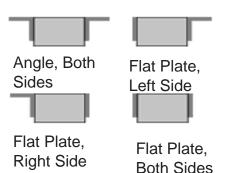
Bumpers may be ordered with angles or flat plates at each er Use a flat plate for mounting bumper next to a dock leveler, o where the space is to tight to allow the use of angles. Note: When using the flat plate, it is welded to the dock.
