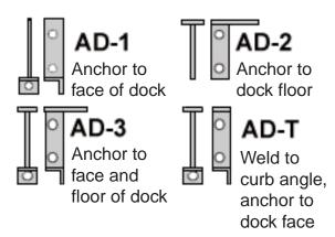
Bumpers may be ordered with angles or flat plates at each er Use a flat plate for mounting bumper next to a dock leveler, o where the space is to tight to allow the use of angles. Note: When using the flat plate, it is welded to the dock.
