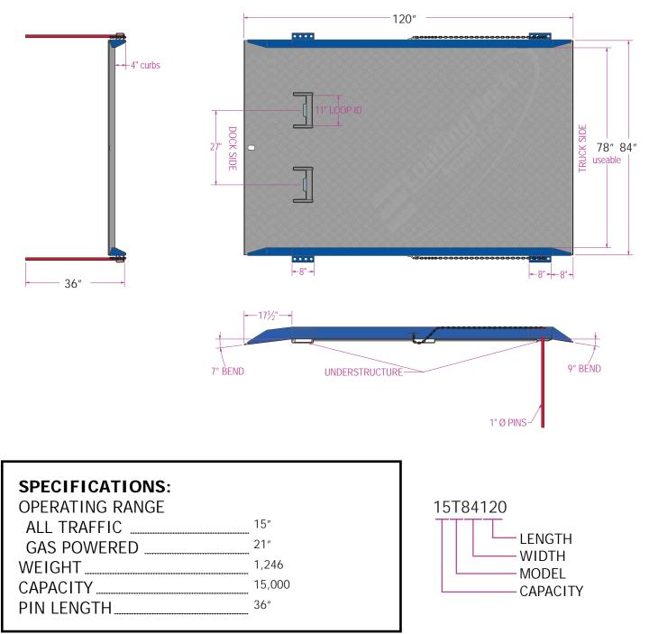
Capacities are based on 3x the carrying capcity of 4 wheeled forklift and four times the capacity of three wheeled forklift; increase to next capacity if used in excess of 8 hours a day.
