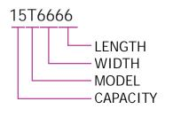
Capacities are based on 3x the carrying capcity of 4 wheeled forklift and four times the capacity of three wheeled forklift; increase to next capacity if used in excess of 8 hours a day.
